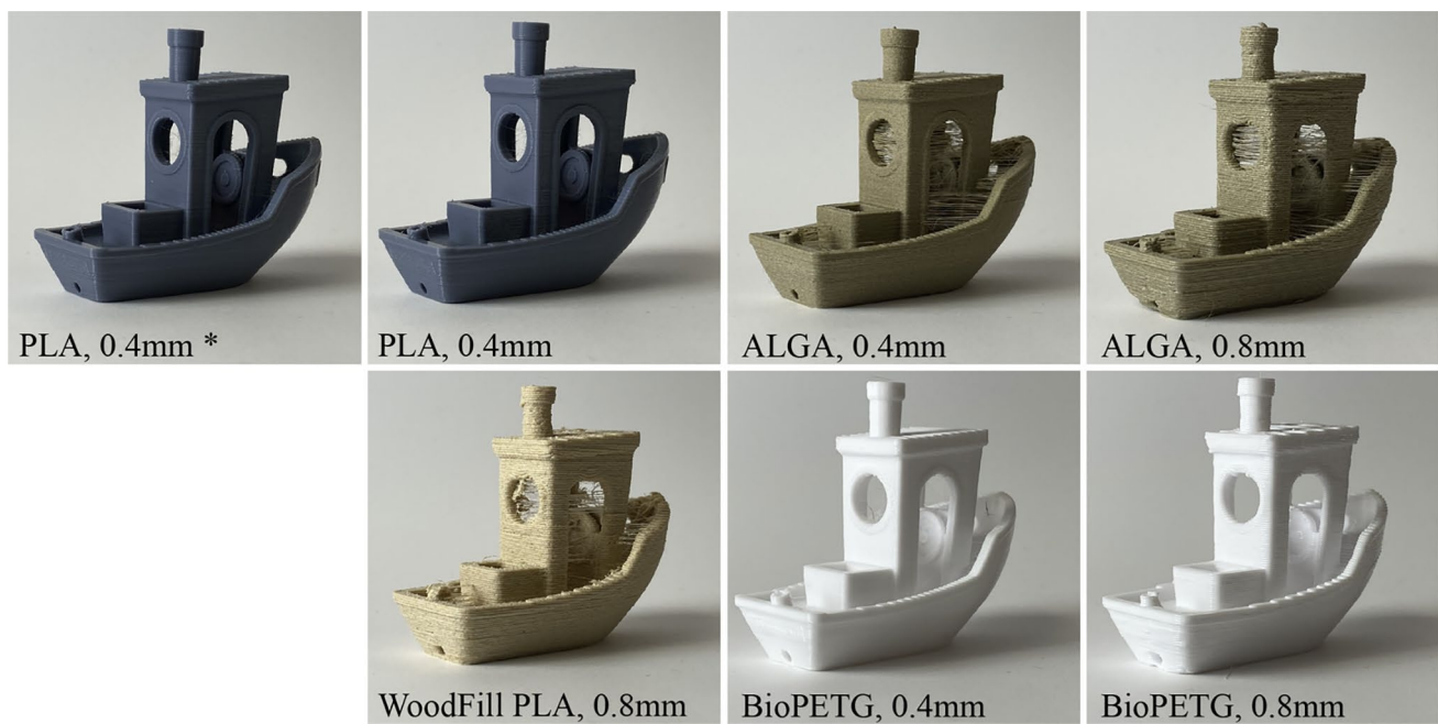
Fig. 6 We deployed our process to produce print parameters for six unique machine, material configurations. We then used those parameters to print the 3DBenchy model [35], a common benchmarking artifact among FFF users and researchers. We include here, one model
